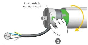
When the drive adapter rotate in a clockwise direction or stop(the black wire and blue wire connect with power), press the setting button in the limit head, the motors will rotate in a clockwise direction
