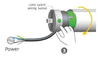
Release the setting button in the limit head
