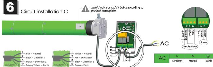
Using special regulator to adjust "+" direction, and rotating white worm when need to increase the up distance
